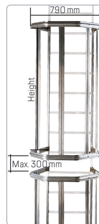
STANDARD HOOP Ladder not included with the standard hoop. Height from 0.62 to 1.46 m, every 28 cm.
