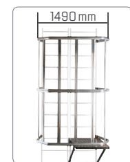
CAGE CHANGE Ladder not included with the cage change. Height 2 m for installations over 8 m. Side walkthrough between straight cages. Non-slip platform. Can be fitted to the left or right. (Ref 09111401)
