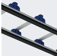
Non-slip rubber strips to protect the roof and ensure greater grip
