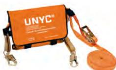
Used to secure horizontal movement over a length of 20.00m. Polyester 35mm strap with two 1m anchor loops and swivel connectors. Ø 19mm opening. Equipped with a double safety lock ratchet attachment that ensures a smooth tension check. Comes with a PVC bag.
