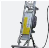
Less handling and reduced risks of theft due to winch being incorporated into the base mast
