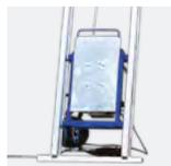
Removable hoist to fit a standard base ladder (no ladder with a special base required) together with an anti-theft system
