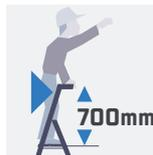
Maximum safety. Guardrail eliminates any risks of tipping over forward
